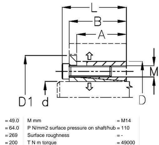
d H8 mm = 200 = 260 D mm Fit tolerance = -F kN torque = 500
